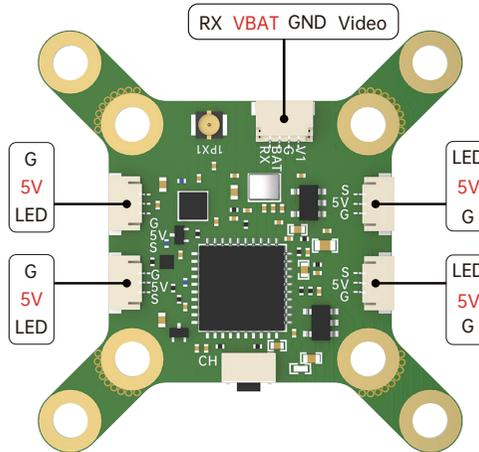
RX: IRC Tramp signal input
